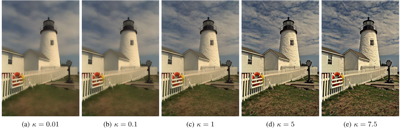
Fig. 4: Effect of varying \kappa for settings r = 11, \epsilon = 0.01, scale = 1 . (a) and (b) Smoothing ( 0 < \kappa < 1 ). (c) Original image ( \kappa = 1 , no filtering). (d) and (e) Sharpening ( \kappa > 1 ).
